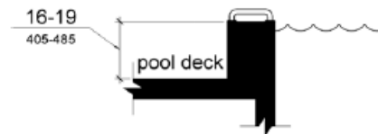
Figure 1009.4.2 Transfer Wall Height
